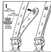
**⚠️ CAUTION** The large disk of the harness fastener is not designed to be inserted through a hole/slot. The small disk is designed to be inserted from the rear of the inside harness strap and then through the rear of the front harness strap.
